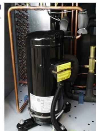
From model ACT 180 on, the type of compressor used is the scroll. Widely used in the air conditioning and refrigeration sectors, the scroll compressor performs well and has low energy consumption. Compression of the refrigerant is achieved by way of two concentric coils: one fixed and the other rotating. The scrolls are wear-resistant, highly reliable and guarantee a high level of noise reduction.
