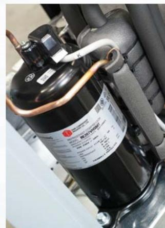
This is a new technology applied to refrigerants as an alternative to the traditional piston compressor. Compression of the refrigerant is achieved by way of interaction between a cylindrical stator and a rotating eccentric nucleus. In this method, the parts which come into contact with one another are wear-resistant and therefore more reliable.
